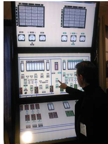
Figure 2: Hybrid simulator developed by GSE Systems for nuclear reactor control rooms: the three boards are scale 1 ontouch screens and all components are virtual.
