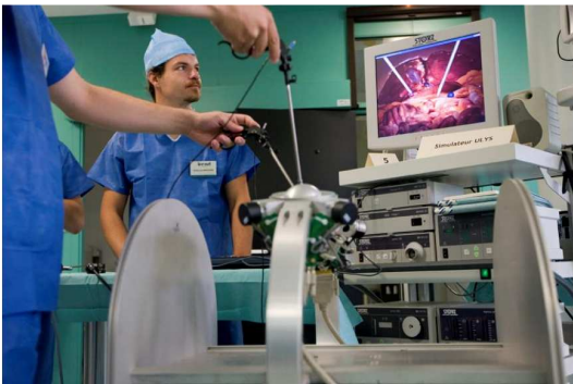
Figure 1: Hybrid simulator ULIS for surgeon training [11] combining virtual scenes inside a patient on the computer screen and real surgery tools with force feedback.
