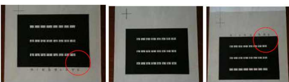
Figure 7a, b & c: Examples of shifting of the mask when using only the middle line.
