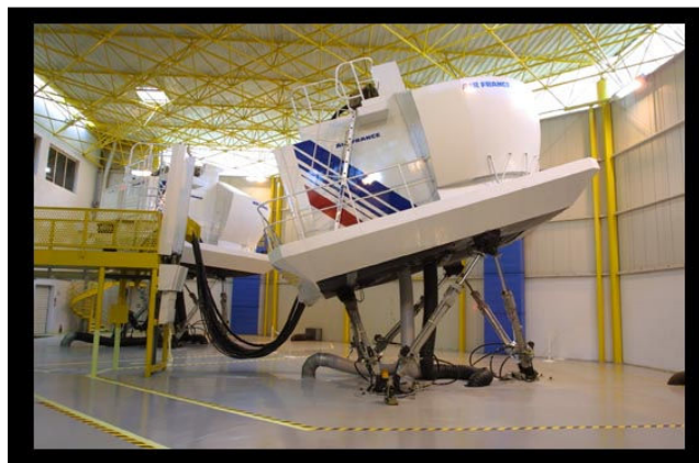
Fig. 1 Example exterior of a Full Flight Simulator of Air France-KLM, Vilgenis training center (Massy-Palaiseau, France)
