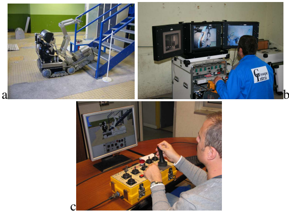
Fig. 4 a) INTRA robot on full scale simulation session, b) INTRA contro panel during training session, c) The virtual simulator for INTRA with virtual images on the control screens generated by the calculation software developed by ITUCR.
