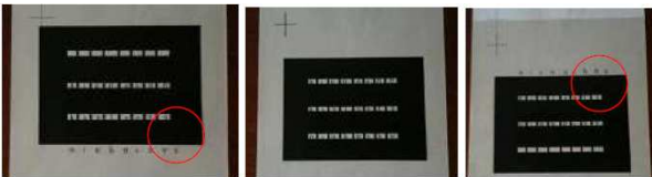
Fig. 5 b & c. Examples of shifting of the mask when using only the middle line.
