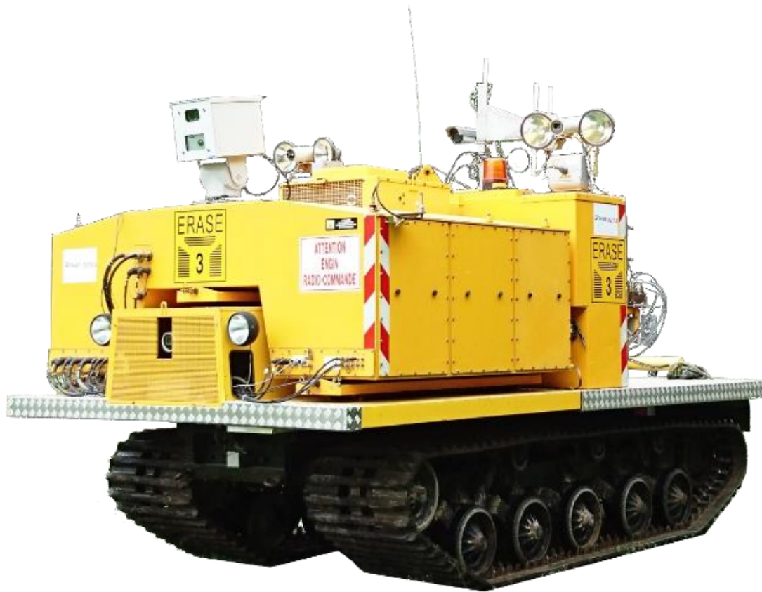
Fig.3: Heavy robot equipped with an articulated arm of several meters for manipulation of equipment outside: ERASE.
