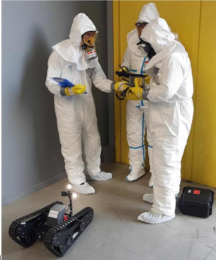
Fig.2 a & b: Pilots equipped with CBRN outfits preparing for remotely operated exploration by ground robot (a) and flying an aerial drone (b).
