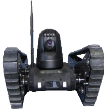
Fig.1: Example of a ground robot for visual and radiological exploration– NERVA XX from NEXTER.
