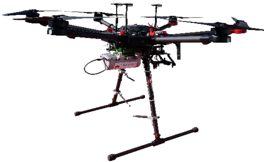
Fig.5: Large wingspan drone, carry 5kg: MATRICE 600 from DJI.
