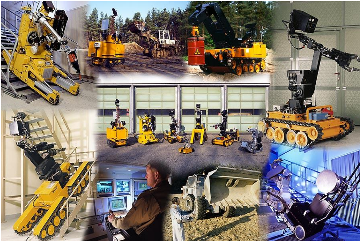
Fig.1: KHG fleet ranging from small inspection robot for pipes with a diameter of minimum 0,2m up to a 25T excavator.
