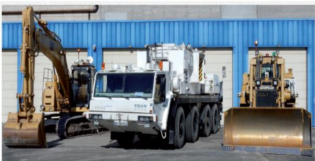
Fig.4 : Teleoperated heavy public work machines: EPELL, EPPB, EBULL.
