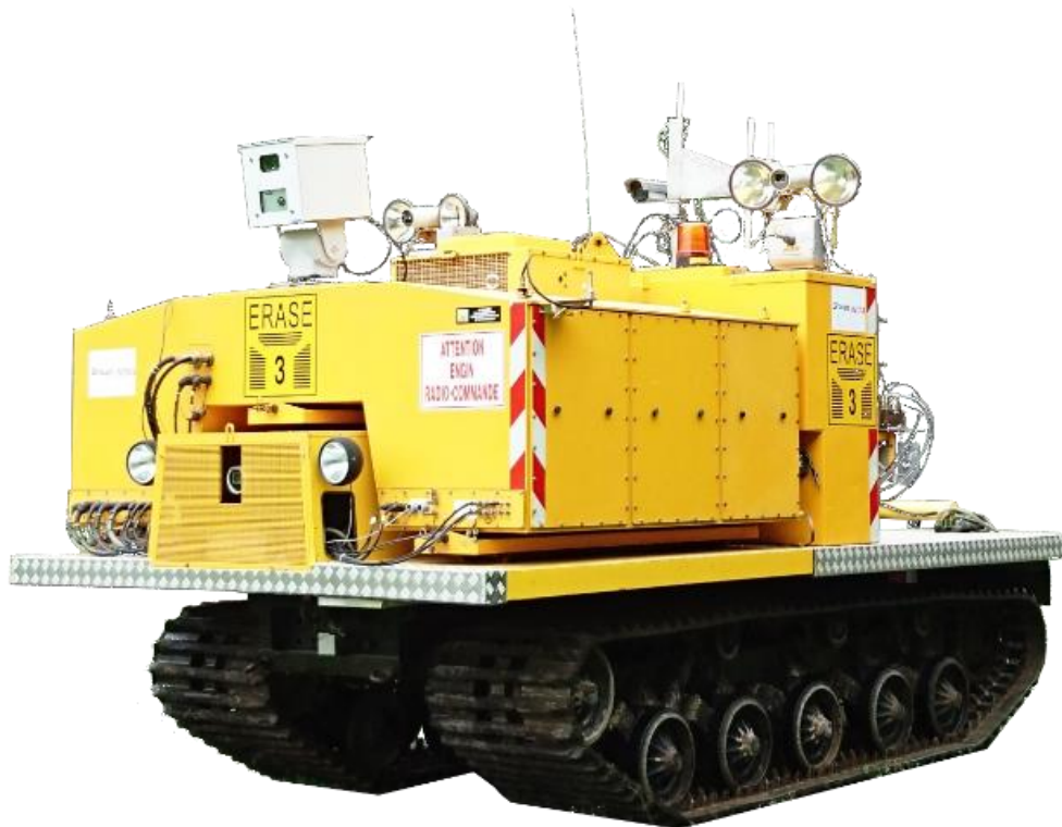
Fig.2: Heavy robot (6T) equipped with an articulated arm of several meters for manipulation of equipment outside: ERASE.
